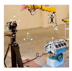
Figure 1: The vision system and the laser tracker groundtruth system.
